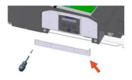
5. Remove the 2 screws and detach the Control Panel and disconnect the mains lead.
