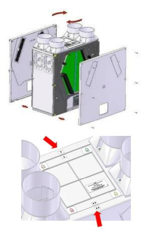
The arrow labels on the top edge of the Covers should be correctly matched to the arrow labels on the top of the Case.
