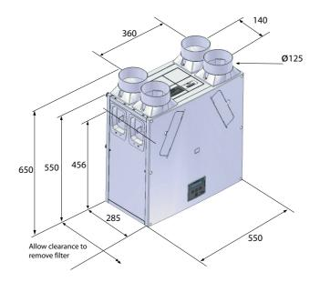
Figure 3: Kinetic E Dimensions
