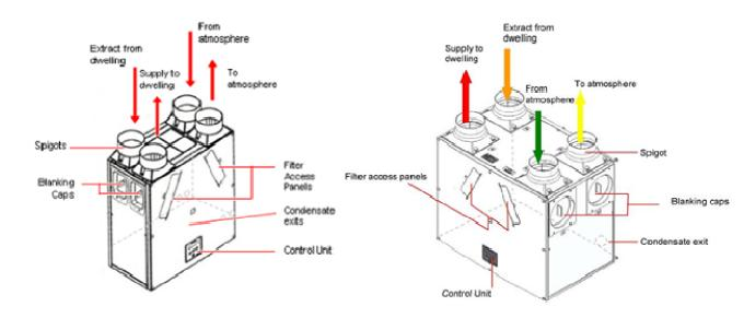
Figure 1: Kinetic E (Front of Unit as supplied)
