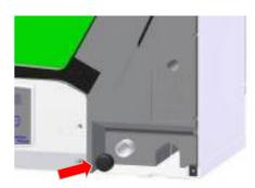
**3.** On the Kinetic E drill a diameter 32 mm whole where shown, right.
