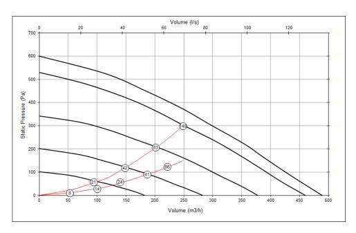
Note: Graph show 2 typical system curves with total unit input power in Watts.
