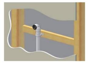
Fit the 180 degree bend supplied to a 22mm diameter x 280mm long condensate pipe with worm drive clip.
