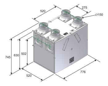
Figure 4: Kinetic Plus E Dimensions
